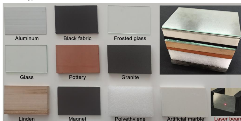
Figure 5. Materials used in experimental studies and sample laser beam on the material(Olgun & Türkoğlu, 2022)
