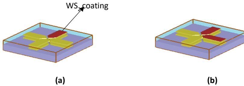
**Figure 5.** (a) Antenna design with one arm of the top antenna layer supported by  $WS_2$  (b) Antenna design with two arms of the top antenna layer supported by  $WS_2$
