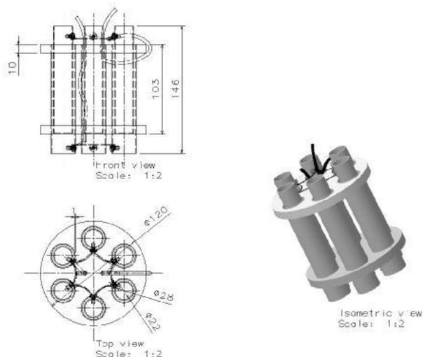
Figure 2. Technical drawing of the electrode design
