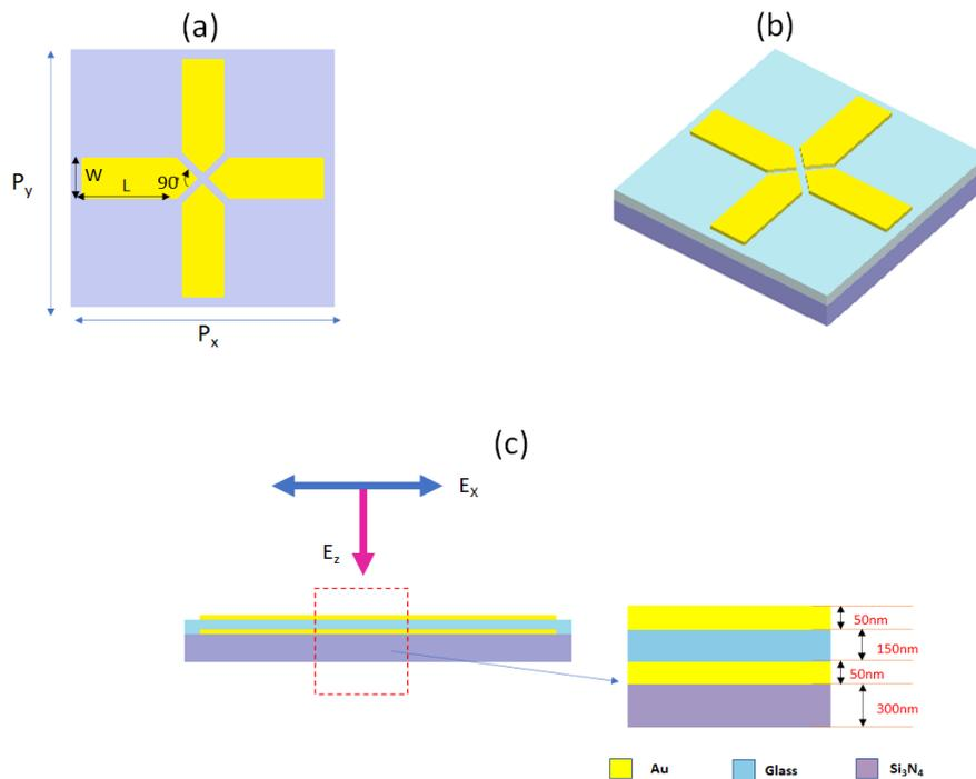
**Figure 2.** The designed basic antenna structure: (a) top view, (b) perspective and (c) side views.
