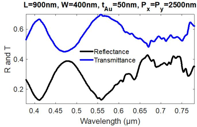
**Figure 4.** Reflectance and transmittance spectra obtained for geometric parameters  $L = 900$  nm,  $W = 400$  nm,  $C = 50$  nm and  $P_x = P_y = 2500$  nm.
