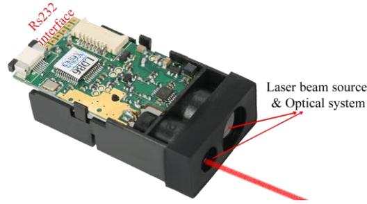
Figure 4. Laser beam source and sensor system
