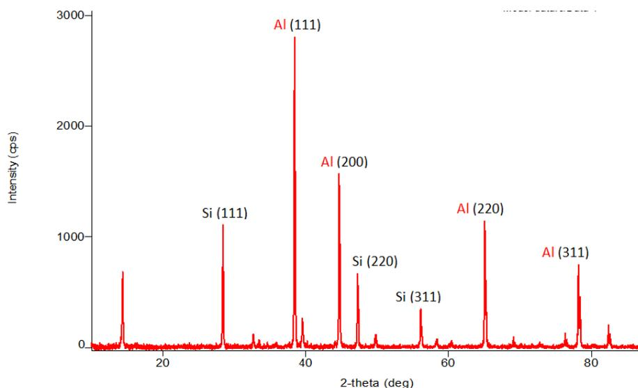
**Figure 2** XRD - MoS<sub>2</sub> and h-BN doped Al-Si%
