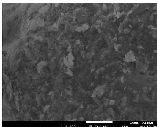
Figure 6 SEM micrographs of worn surface for nanocomposite with 4wt% (MoS<sub>2</sub>) nanoparticles under a normal load (2.5N); at 2000x.
