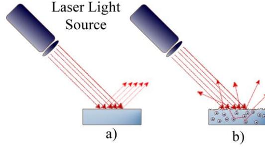
Figure 2. Laser beams and reflection types a) Specular reflection from a smooth surface b) Diffuse reflection and subsurface scattering from a rough surface
