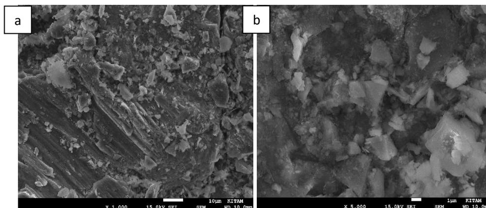
**Figure 5** SEM micrographs of worn surface for hybrid Nano composite with 4wt% (MoS<sub>2</sub>+ BN) nanoparticles under a normal load (2.5N); **a**) at 1000x, **b**) at 5000x.
