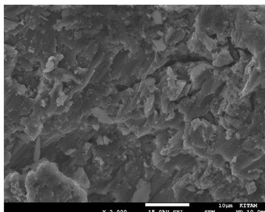
Figure 7 SEM micrographs of worn surface for nanocomposite with 4wt% (BN) nanoparticles under a normal load (2.5N); at 2000x.
