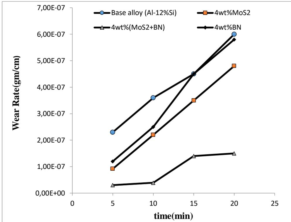
Figure 3 Comparison between wear rates of base alloy, hybrid nanocomposite with 4wt % (MoS<sub>2</sub>+BN), nanocomposites with single addition 4wt% MoS<sub>2</sub> and 4wt% BN as a function of time.
