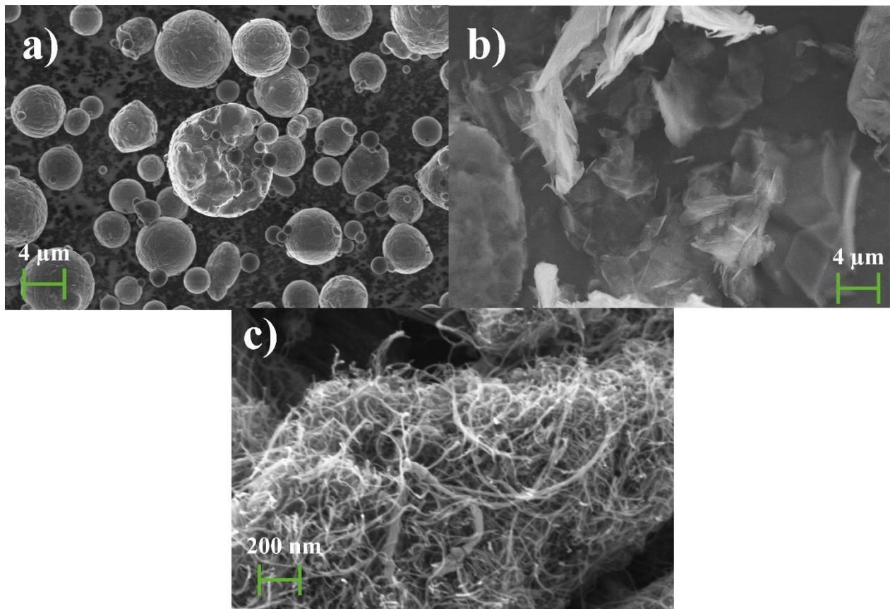
**Figure 1.** Matrix and reinforcement powders a) Al6061 b) GNP c) MWCNT
