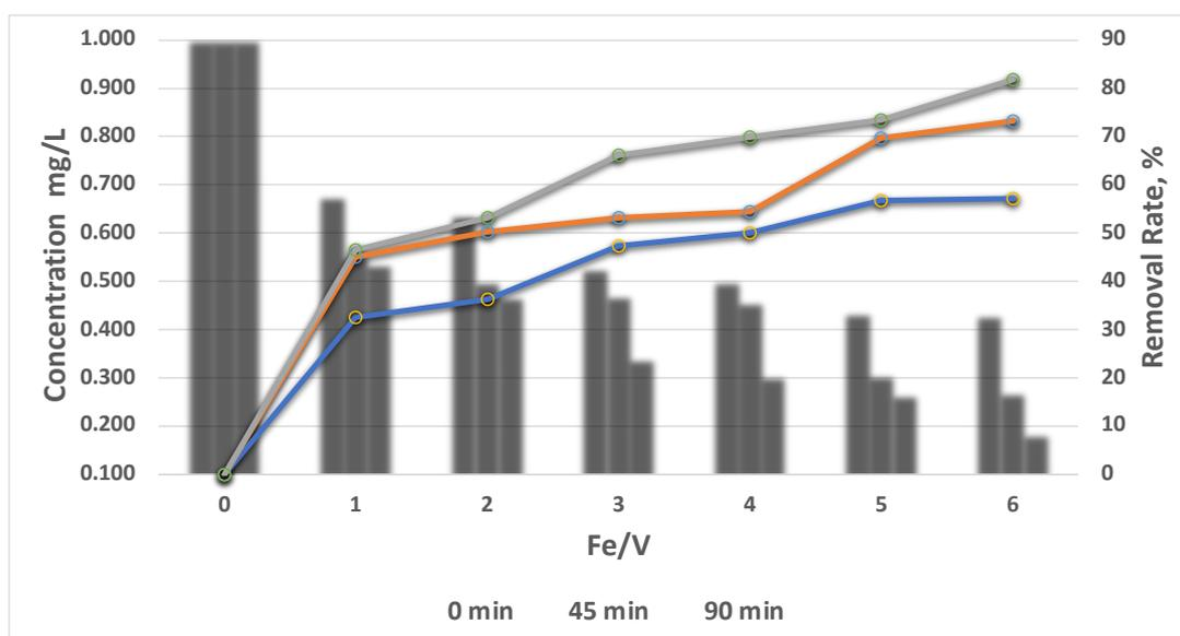
Figure 3 Effect of Fe/V dose on the removal of Vanadium with FeCl<sub>3</sub>
