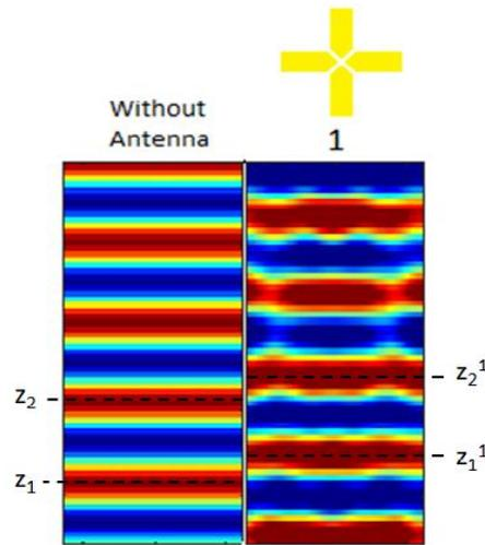
**Figure 7.** Determination of phase difference from field distributions caused by source only and basic antenna structure
