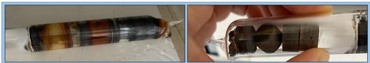
Figure 4. Composite materials sintered in a quartz tube
