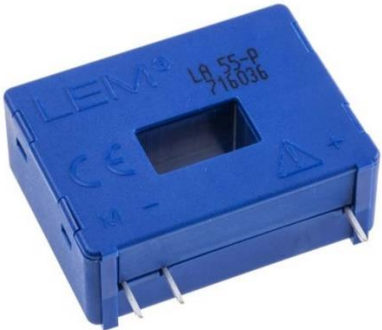
Figure 3. LEM-LA55P current transducer and its connection
