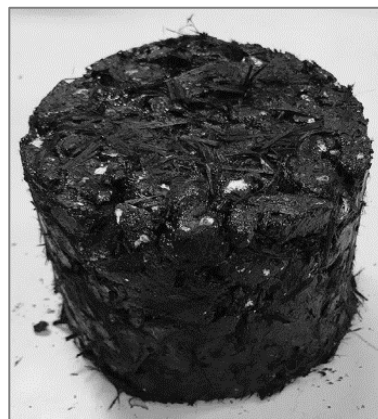
Figure 2. An Asphalt Sample with a Heterogeneous Structure Due to Its High Fiber Content (Cetin et al., 2021)
