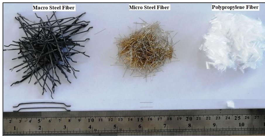
Figure 1. The pictures of macro and micro fibers.
