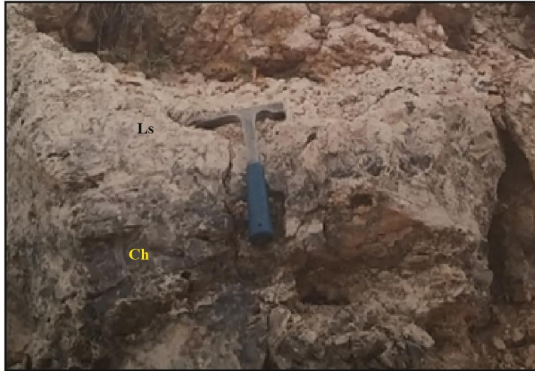
Figure 7. The cherty (Ch) limestone (Ls) observed in the Uzunçarşidere Formation (east of Dedeçanı Tepe). Scale (hammer length: 28 cm)
